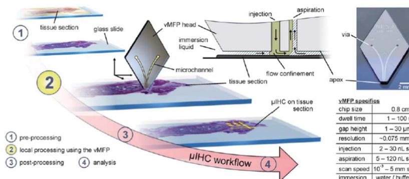
**Fig. 2** Concept of micro-immunohistochemistry using a vertical microfluidic probe (vMFP) and a list of typical experimental parameters. Figure reprinted with permission from the Royal Society of Chemistry from Lovchik *et al.*<sup>6</sup>
